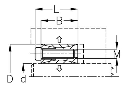
$\begin{array}{lll} \text{B mm} & = 33 \\ \text{d H8 mm} & = 120 \\ \text{D mm} & = 165 \\ \text{Fit tolerance} & = \text{Aksel k11-h11, Nav N11-H11} \\ \text{F kN torque} & = 132.0 \\ \text{L mm} & = 45 \\ \text{M mm} & = \text{M12} \\ \text{P N/mm2 surface pressure on shaft/hub} = 51 \end{array}$
